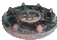
2nd stage water-cooled valve after 800 hours
