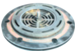
3rd stage air-cooled valve after 2,500 hours
