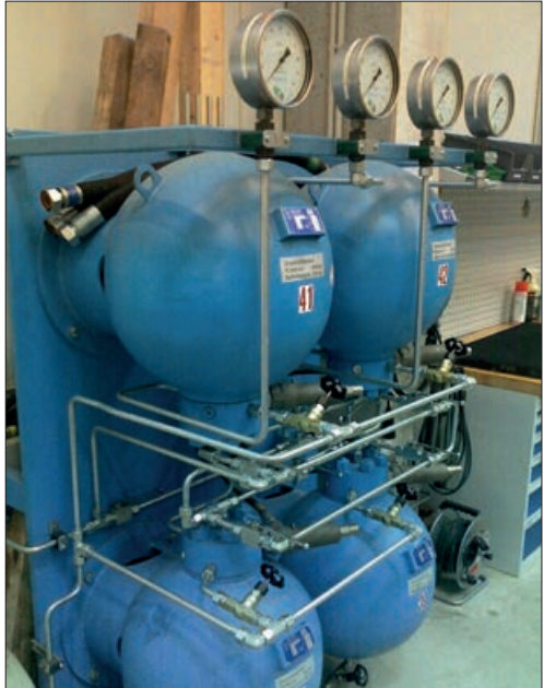
Fig. 12: High-pressure vessel to 600 bar
