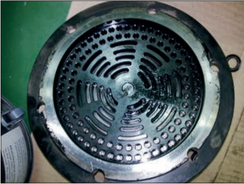
Fig. 29: Carbon build-up on a valve from oil residue and overheating
