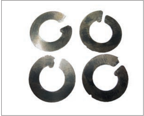
Fig. 22: Valve spring failures
